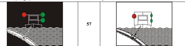
Article 3.25, paragraph 1, letters a and b: Floating equipment at work and vessels carrying out work or sounding or measuring operations; fairway clear on one side.
