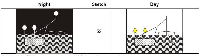
Article 3.24: Stationary vessels engaged in fishing with nets or poles.
