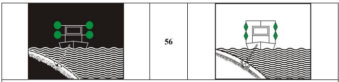
Article 3.25, paragraph 1, letter a: Floating equipment at work and stationary vessels carrying out work or sounding or measuring operations; fairway clear on both sides.
