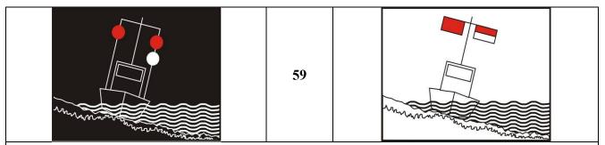
Article 3.25, paragraph 1, letters c and d and paragraph 4: Floating equipment at work and vessels carrying out work or sounding or measuring operations and grounded or sunken vessels; protection against wash; fairway clear on one side
