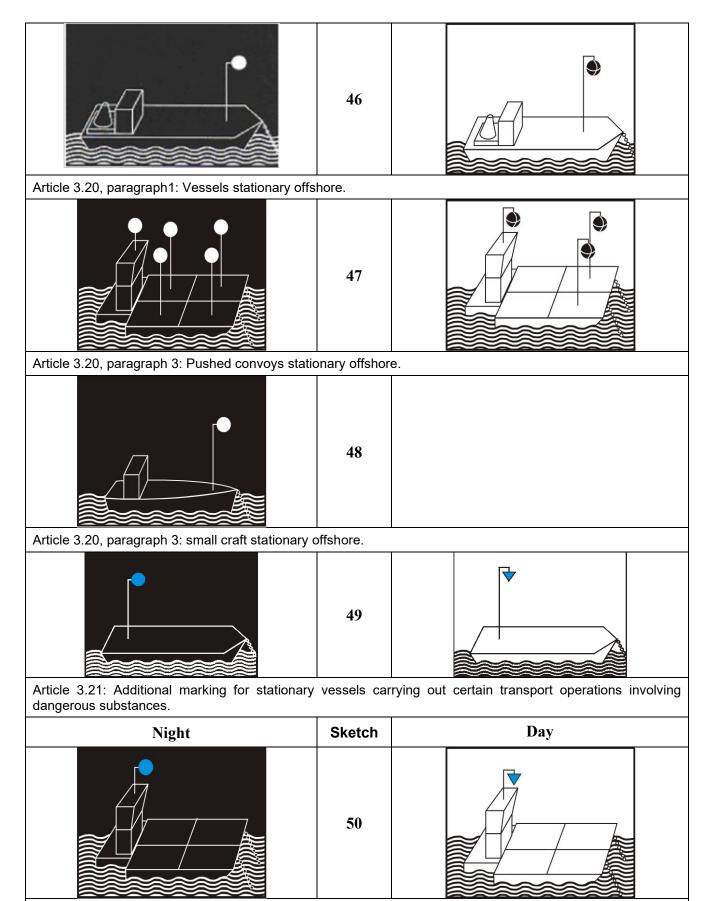
Article 3.21: Additional marking for stationary pushed convoys carrying out certain transport operations involving dangerous substances.
