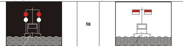
Article 3.25, paragraph 1, letter c and paragraph 4: Floating equipment at work and vessels carrying out work or sounding or measuring operations and grounded or sunken vessels; protection against wash; fairway clear on both sides.
